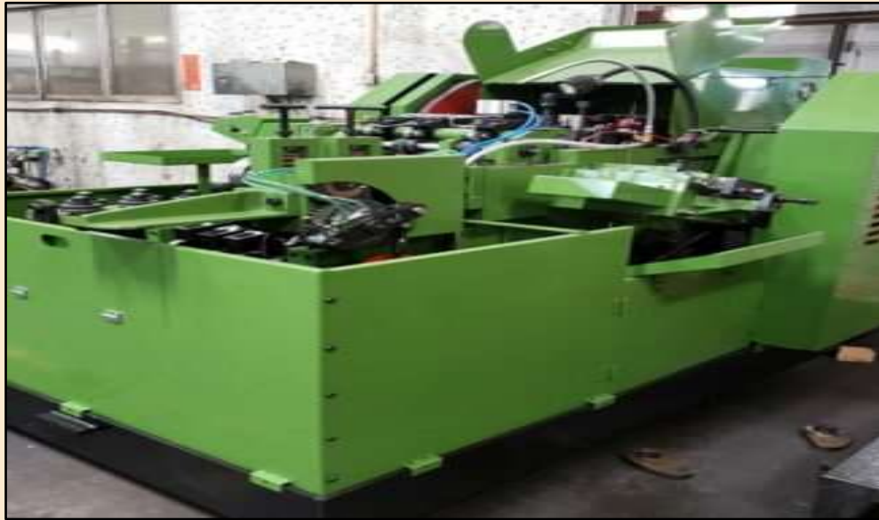
6 station cold forging machines with ranges from M4 to M18
