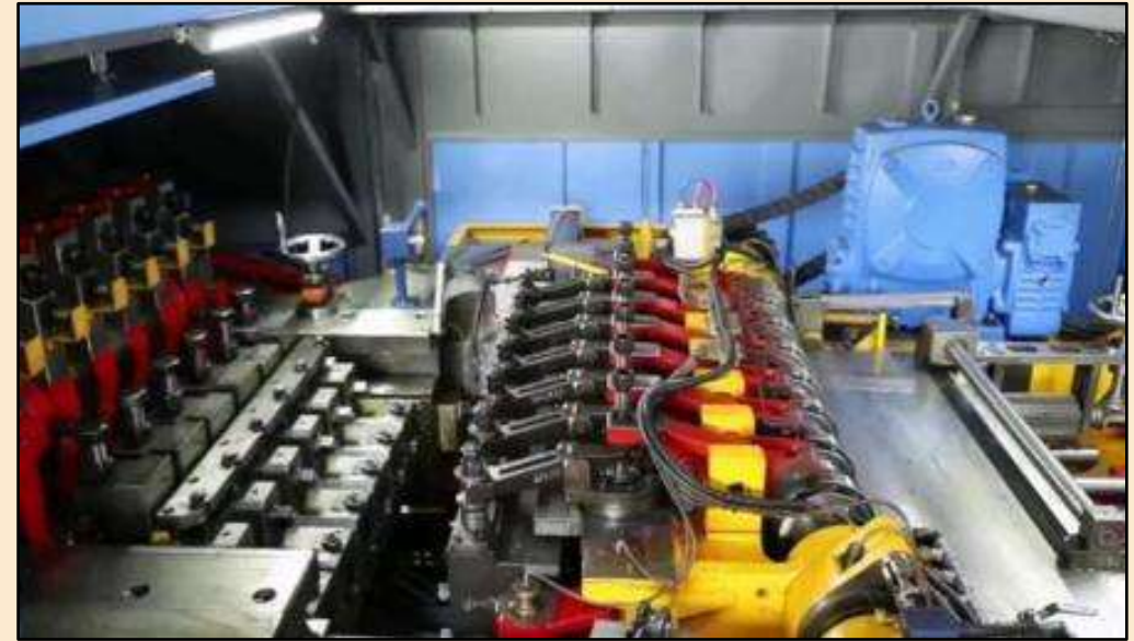
6 station cold forging machines with ranges from M4 to M18
